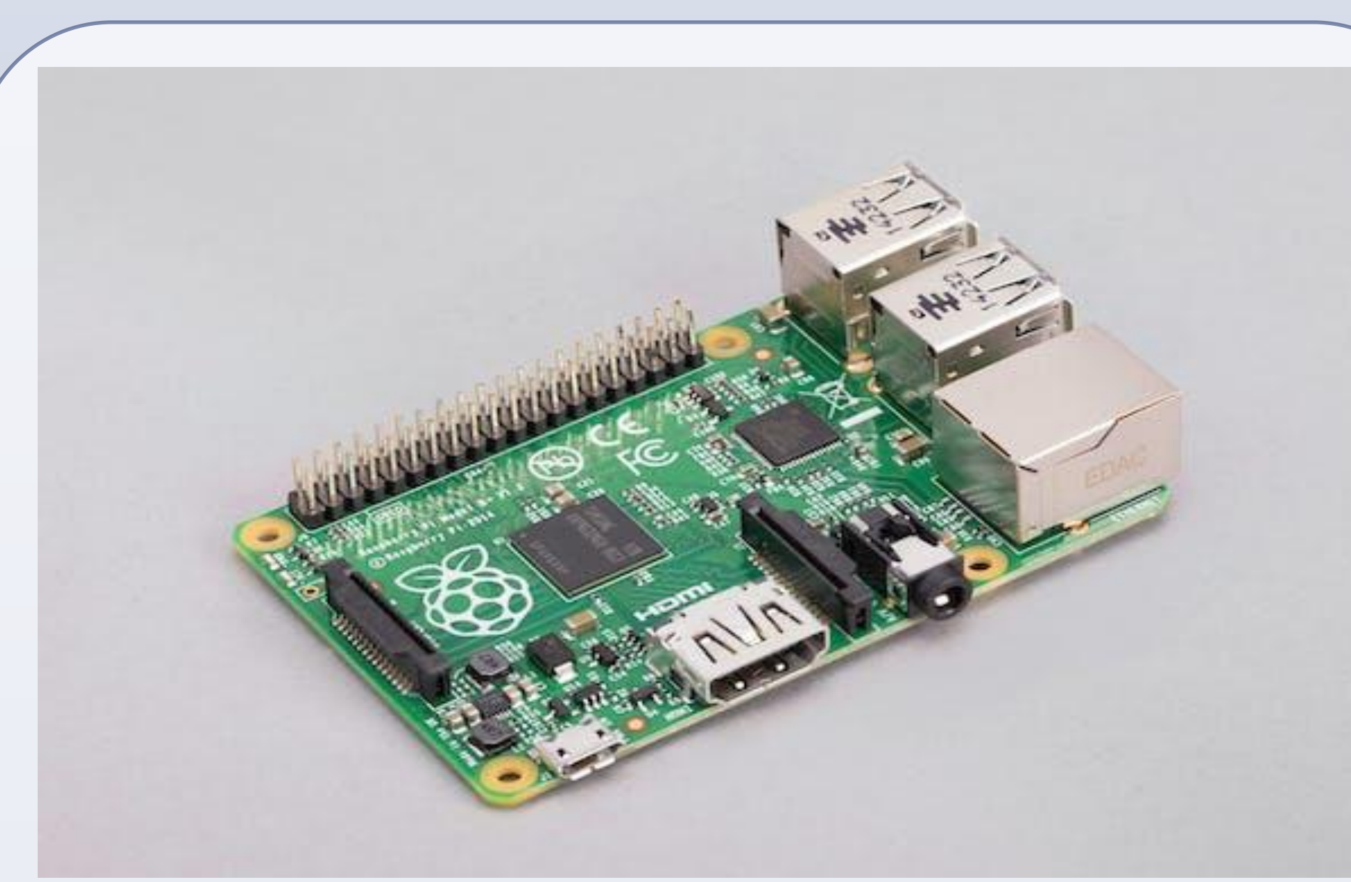
Fig. 6: Raspberry Pi device that is necessary to use Octoprint.
