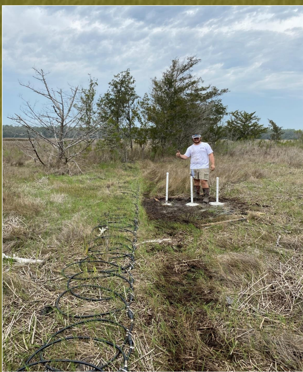
Figure 4. Groundwater wells after installation (right), short transect electrode and cable array (left).
