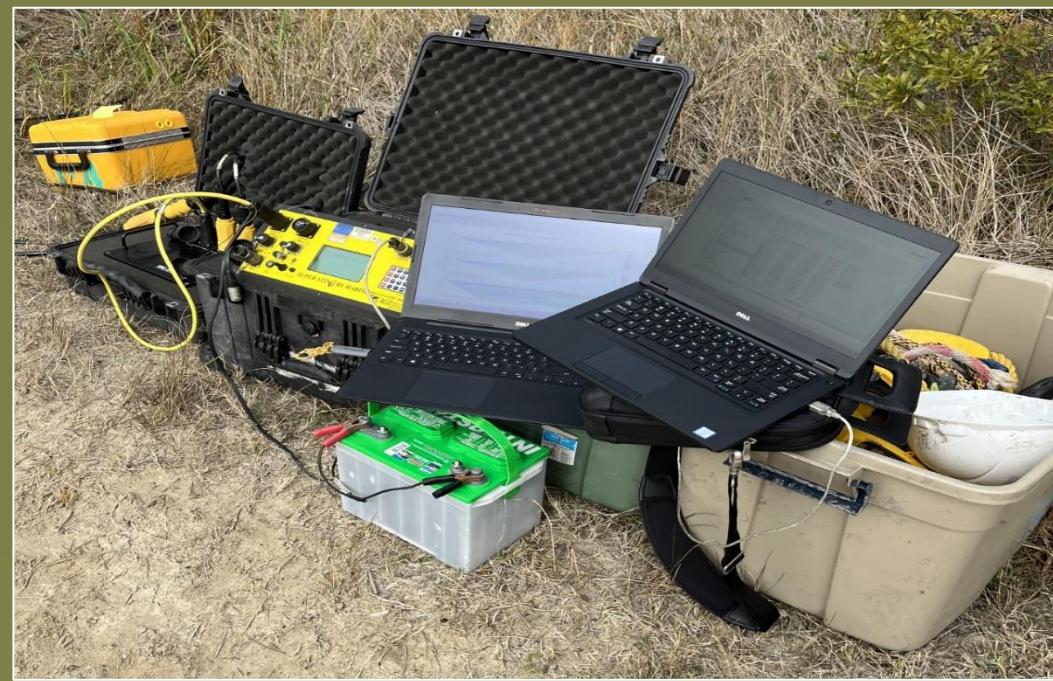
Figure 1. Typical instrument package for electrical resistivity surveys including SuperSting R8 head unit, switchbox, imaging processing laptops and remote power.
