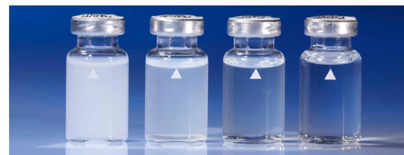
Examples of high turbidity to low turbidity (In most cases, the clearer the water, the lower the turbidity levels)
