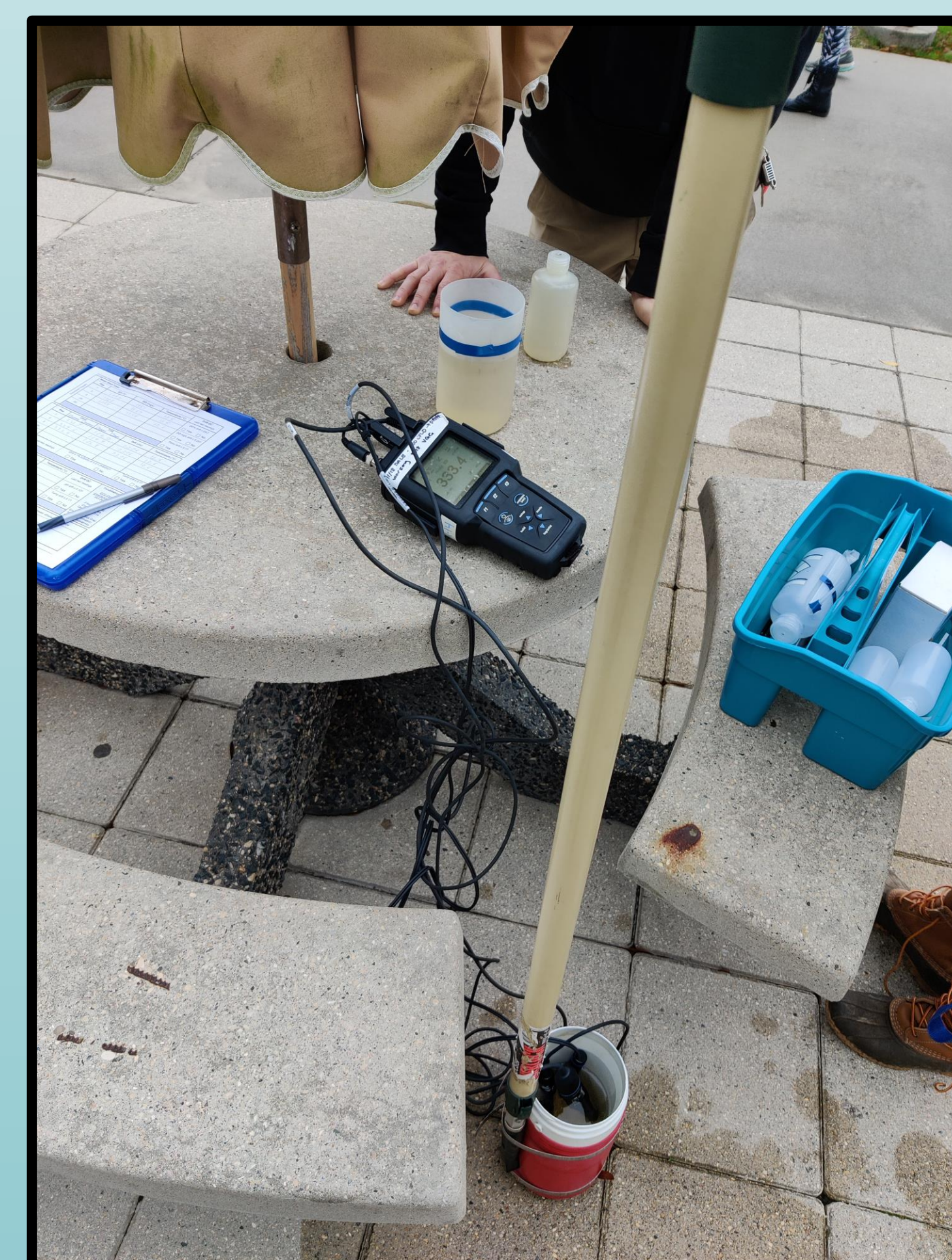
Figure 2: Tools used for data collection (Orion™ A329 multimeter, extendable pole with a ~1-quart bucket fixed to it, & data collection sheets).
