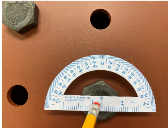
Figure 7. The manually measured bolt rotation angle using a protractor
