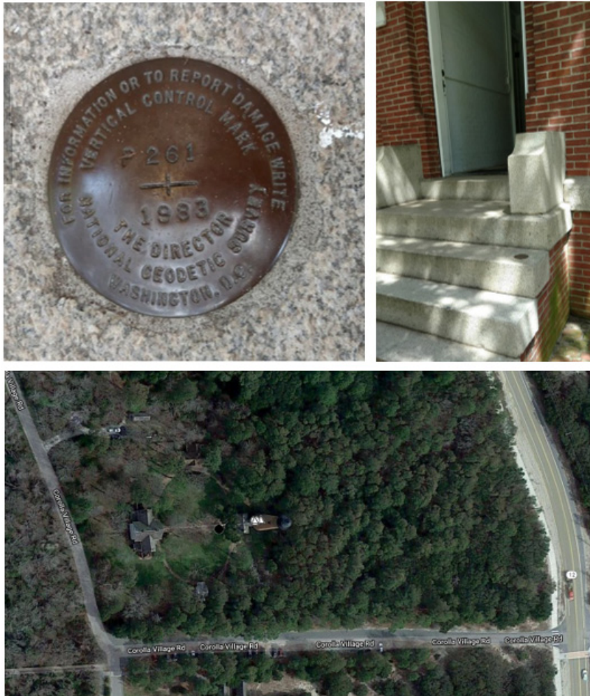
Figure 05. Photographs of the benchmark used to set vertical and horizontal datum for control baseline. Reference for differential level run.
