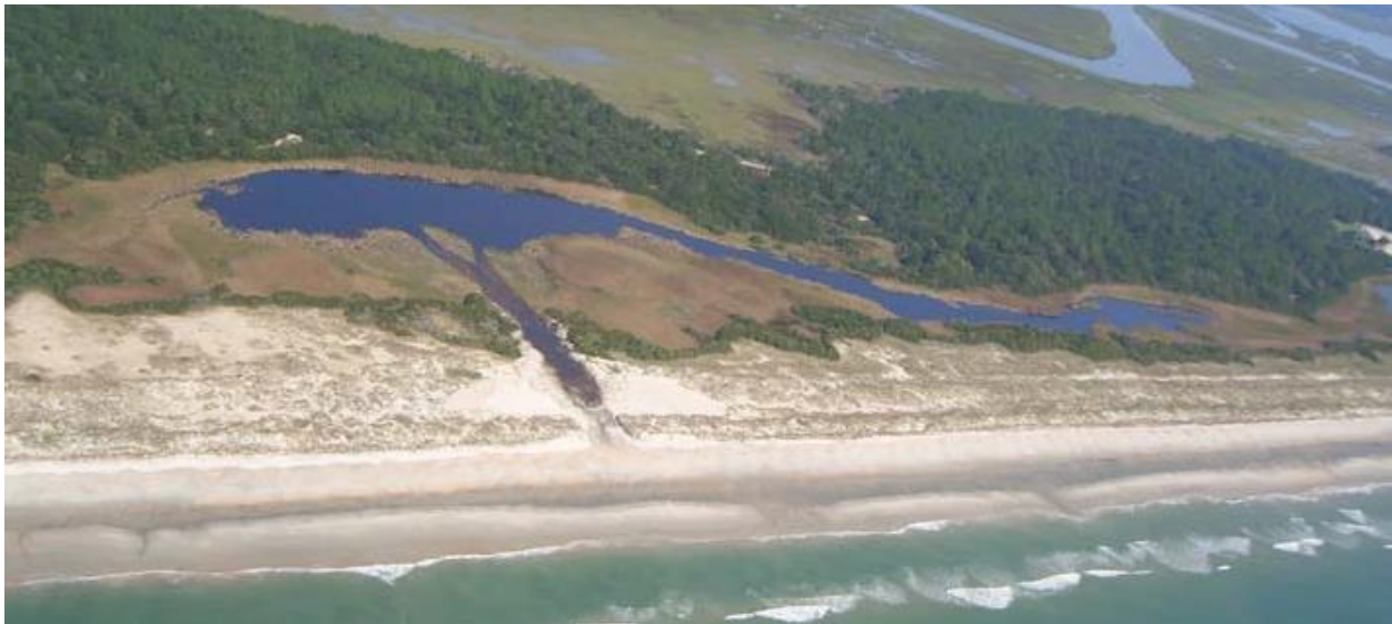
Figure 2 Aerial photograph of Sandpiper Pond (Huntington Beach State Park, Georgetown County, South Carolina) after cutting of the ocean tidal channel (from Tosso 2006).
