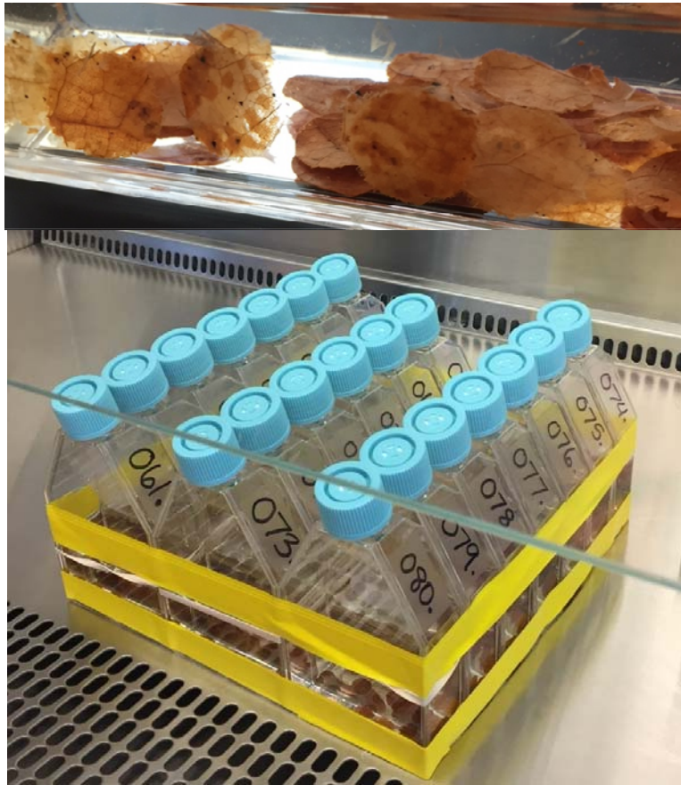
Figure 1. Laboratory microcosms (tissue culture flasks) containing naturally colonized tulip poplar leaf disks with nutrient solution that were incubated at 5 temperature treatments (4-20°C) for 28 days.
