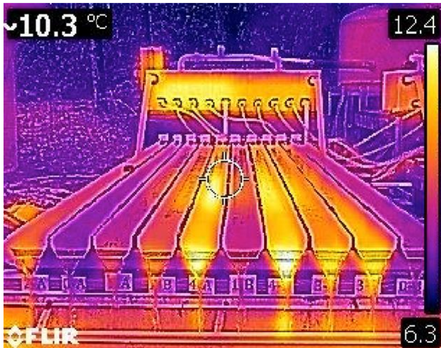
Figure 2. Top panel: Experimental set up with 20 streamside channels (5 temperature treatments \times 4 replicates). Bottom panel: 10 of the streamside channels (two replicates of each temperature treatment: 0 (ambient control), +1, +2, +3, and +4°C) showing \pm 1^\circ\text{C} differences in temperature (thermal imaging); photo credit: J. Benstead, University of Alabama.
