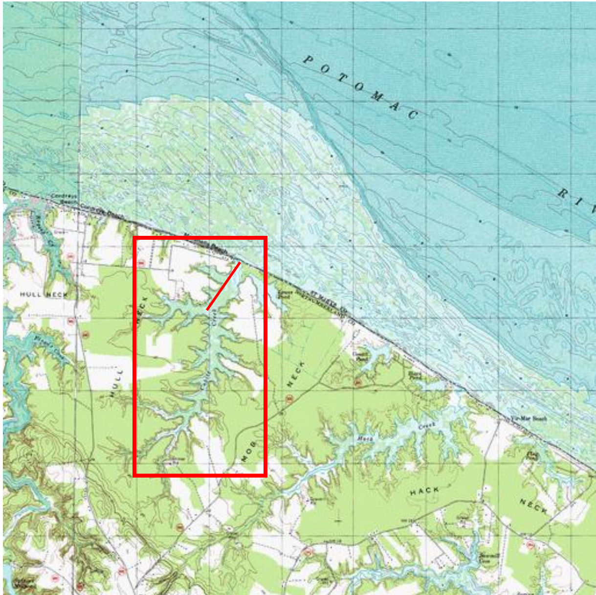
Figure 1: The USGS 1973 topographic map of Burgess, Virginia shows the elevation range of one to five feet and a mean sea level of three feet. The samples were taken along the red transect.
