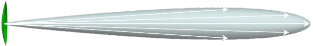
Figure 2: Parabolic radiation pattern produced by a dish antenna (reproduced here from Wolff, 2009).
