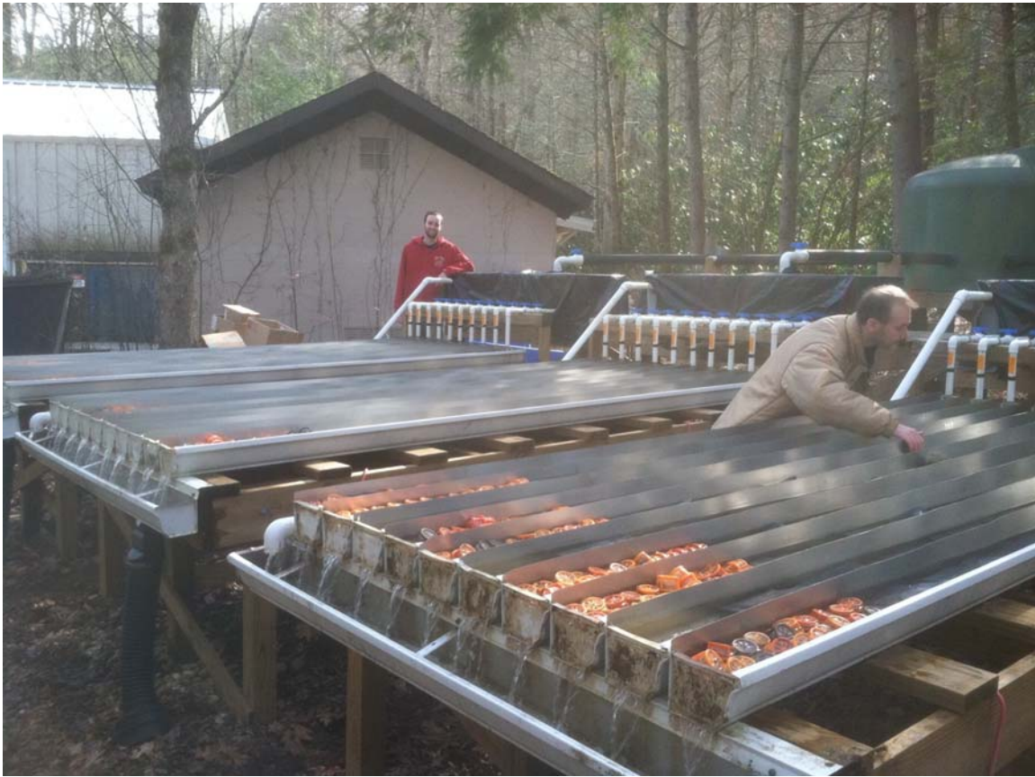
Figure 1. Thirty streamside channels fed with water pumped from the Shope Fork at Coweeta Long Term Ecological Research site in North Carolina used for decomposition experiments under varying dissolved nutrient concentrations.
