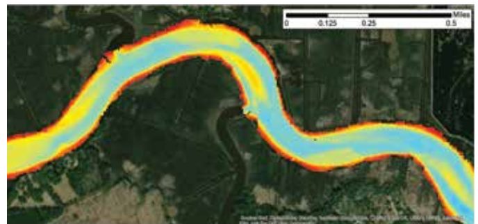
Figure 3: Bank-attached shoals at the lee sides of inner bend sides, suggesting the importance of the ebb flow for net sand transport down the stream.
