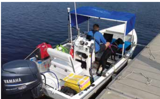
CCU's small boat is equipped with sonar for mapping the Sampit River.
