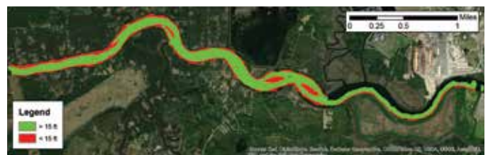
Figure 5: Navigability of the Sampit River where green indicates water depths greater than the required commercial 15 ft. (5 m.) and red shows access limits for barges ( \leq 15 ft. of water depth).
