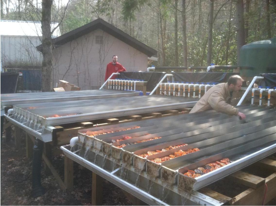
Figure 1. Thirty streamside channels fed with water pumped from the Shope Fork at Coweeta LTER site in NC used for decomposition experiments.
